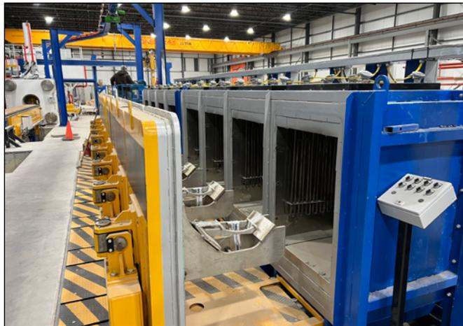
Figure 2. Thermally efficient die ovens.
