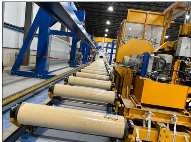
Figure 3. Following the press exit is the BICS quenching system with a double runout table.
