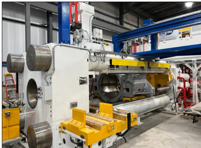
Figure 1. The new 44 MN, 10/12 inch extrusion press in the process of being installed.
